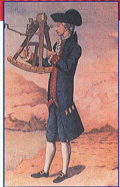
Here, a naval officer uses a sextant, which replaced the astrolabe in measuring the height of the stars above the horizon.
